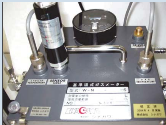
● Ptセンサ (ガス温/液温測定用) Pt sensor(Measurement for Gas temperature/ liquid temperature)
