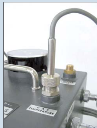
● Ptセンサ (ガス温/液温測定用) Pt sensor(Measurement for Gas temperature/ liquid temperature)
