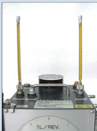
● 温差補正計 (ガス温/液温測定用、40°C) Temperature compensator for percent scale (for Gas temperature/for liquid temperature 40°C)
